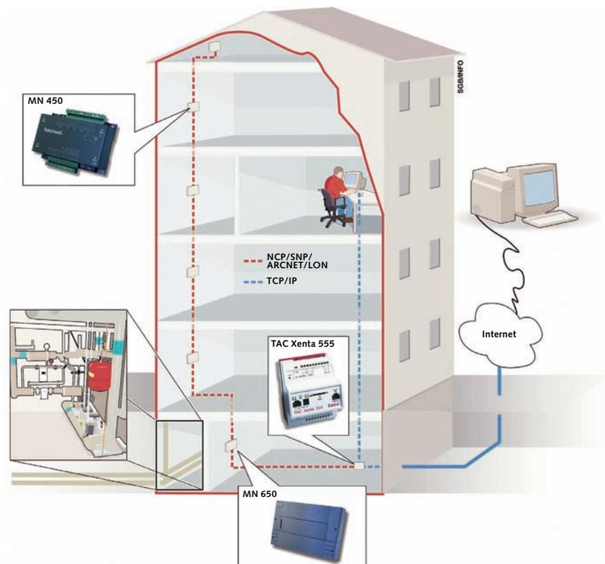
The Xenta 555 allows an operator to easily view and control the devices in a Micronet network via the Internet or a local intranet.
